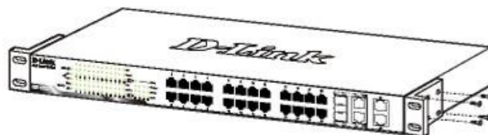
Figure 2.2 – Attach the mounting brackets to the Switch
